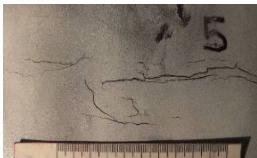
Figure 7. Cracks at the surface of parent material of the anchor of breeches pipe no.1.
